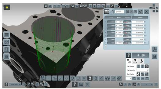
CAD has traditionally added complexity to CMM programming. The optional TouchCAD module of TouchDMIS simplifies CMM programming and introduces touch screen manipulation of the CAD model using gesture commands.
