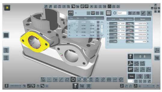
Selection of the Tolerance Button launches the Tolerance Table Window and displays default tolerances imported at TouchDMIS start-up. The Tolerance Window displays tolerances for Features | Geometry | Angles & Lengths. Table selection is via Flip Buttons which 'flip' the Window to the selected table. To tolerance a Feature select a tolerance for the required parameter from the table; a graphic displaying deviation reports actual v tolerance result.
