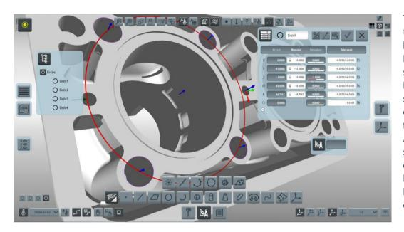
The Construction Professor on the Construct Toolbar is launched by default and the Result Window opened upon selection of the Construct Button; a dynamic toolbar showing available construction options for selected measured features is displayed. A graphical image of the selected construction feature is displayed offering One Touch Feature construction and the Feature result displayed in the open Result Window.
