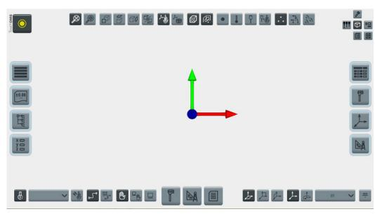
The minimalistic user interface of TouchDMIS has been ergonomically developed to provide maximum productivity for both novice and expert CMM user and utilizes the latest Touch Technology platforms. TouchDMIS incorporates floating toolbars to maximize the graphics area with the principle software functionality accessed via eight large Function Buttons. TouchDMIS has no drop-down menus, no stacked toolbars, and functionality is simply accessed with a single Touch.
